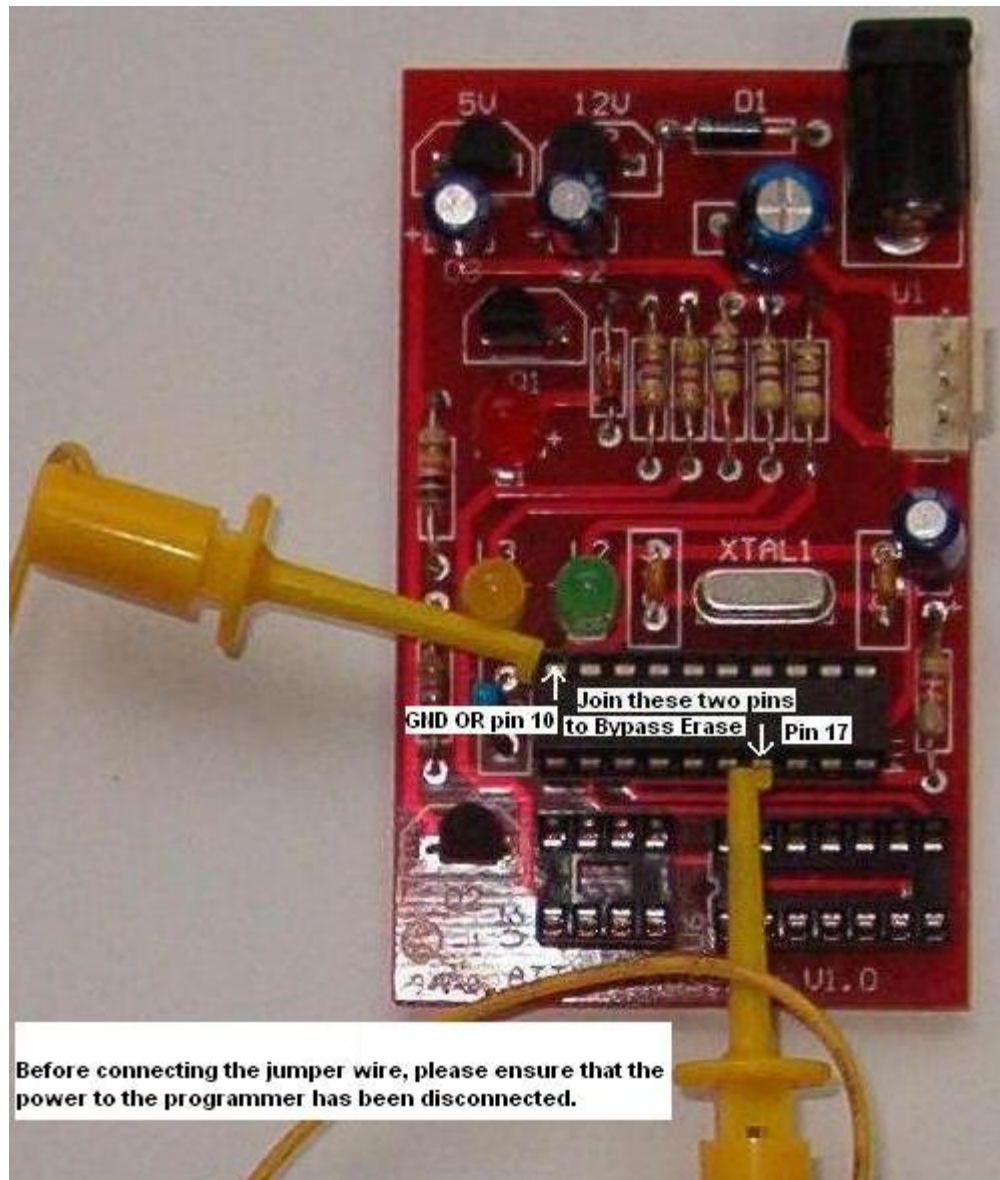
Fig. 3. Connect a jumper wire before the programmer is powered up, in order to ByPass the erase function. This will preserve the code in devices where the lock bits have not been programmed.
