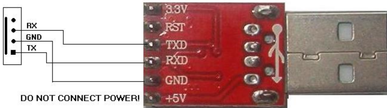
Fig 2. Connecting the Programmer to the Computer's USB Port
