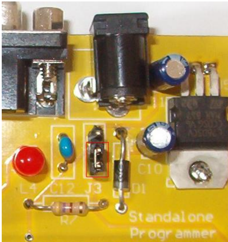
Fig 3. Take power from target 3 - 5 V.
