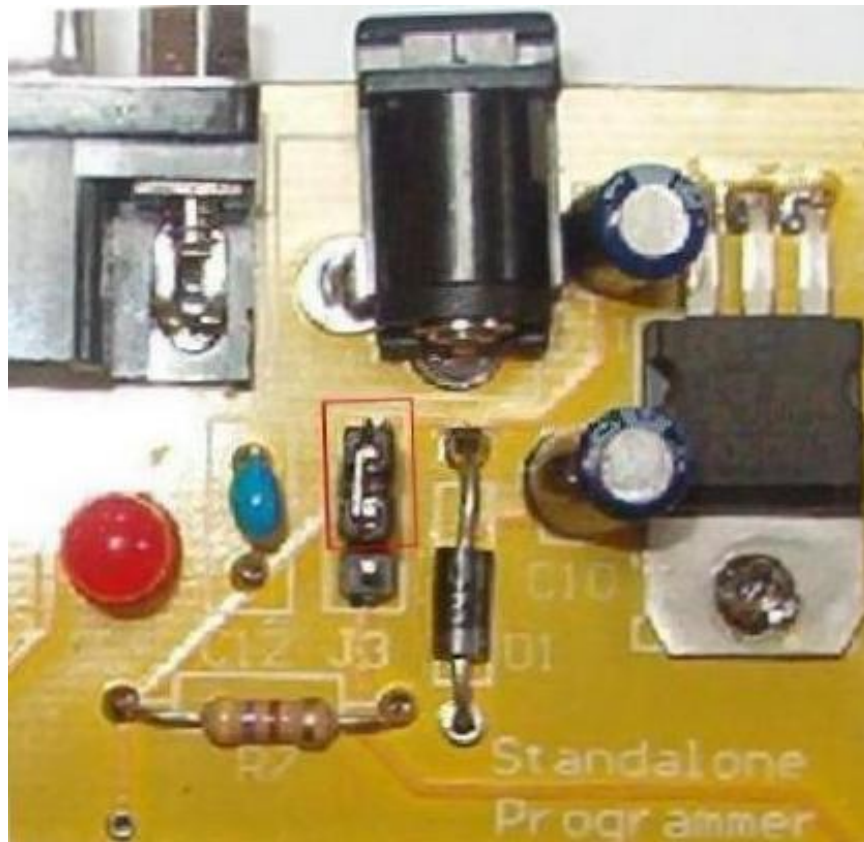
Fig 2. Use programmers own 5V power supply.
